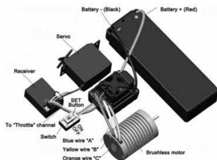
"+" and "-" wires of the ESC are connected with the battery pack, and #A, #B and #C are connected with the motor wires. The "SET" button is used for programming the ESC.
